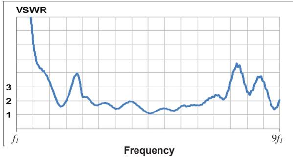
Fig. 6. Measured VSWR for the case of broadside scan.
