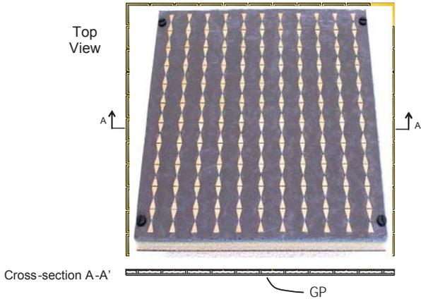
Fig. 1. Top and cross-sectional view of a planar TWA array.
