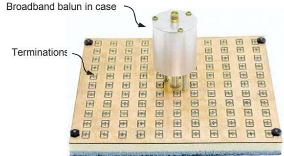
Fig. 5. Back view of an SEG model showing balun feed for center element and resistive terminations for each array element.
