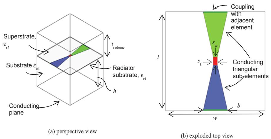
Fig. 3. Unit cell of planar TWA array with planar bowtie elements: (a) perspective and (b) exploded top views.
