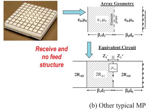
Fig. 2. Comparison of equivalent circuits for a center array element: (a) planar TWA array, (b) other typical MPPA.
