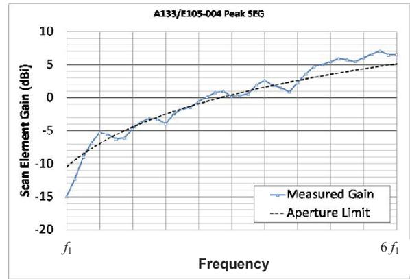
Fig. 8. Measured peak gain per element vs theoretical maximum of an SEG model.
